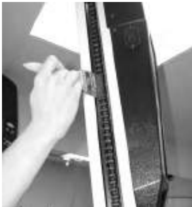
Using a toothbrush, or firm paint brush this is the ONLY place you will use grease on the VersaClimber.
