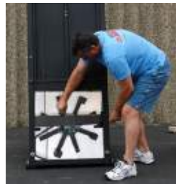
12. Wind 3 turns of the cord around the shaft above the flat washer attached to the bottom of the shaft. For detailed instruction please call us at 1.800.237.2271
