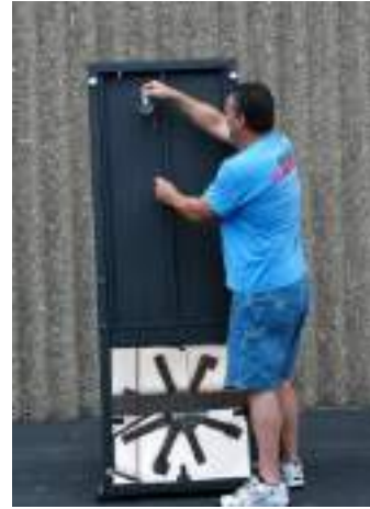
10. Attach the rewind Pulley, located under the housing enclosure, to the hook located in the far corner, under the platform.
