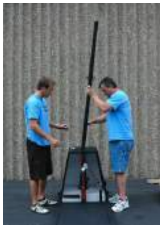
14. Insert the vertical mast into the housing with the mast tilted forward towards the platform.
