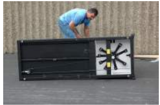
To access and change fly-wheel weights Lean unit over onto side.
