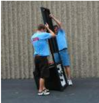
8. Insert the platform into the MV 2 enclosure until the bolt holes on the bottom of the platform are in alignment on either side of the machine.
