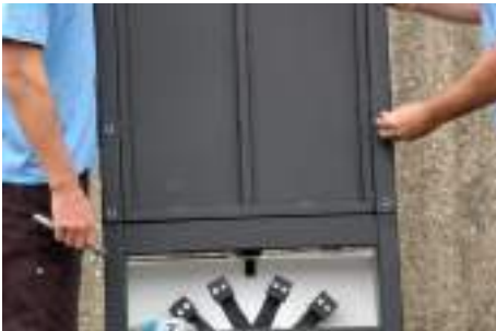
9. Use four 3/8" x 1 1/4" bolts and four 3/8" lock washers and securely tighten deck to housing.
