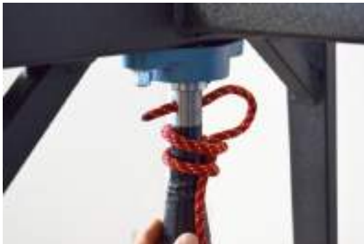
10. With end of rope underneath two loops, feed tip of rope through hole at the top of the cone.
