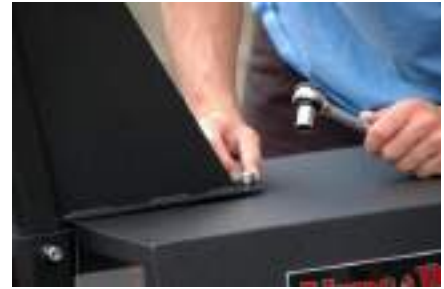
16. Use a 3/8-16 nut to secure the mast to the top of the housing cover.
