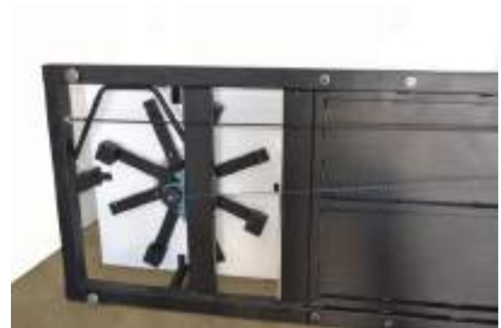
After appropriate fly-wheel weight has been determined (see page 15). Securely tighten block weights.
