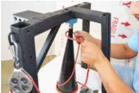
9. At top of cone, loosely wrap rope around twice. Next, push end of rope up underneath.
