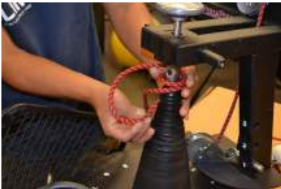
11. After two wraps around cone, thread the rope underneath the looped rope that is lying against the cone.
