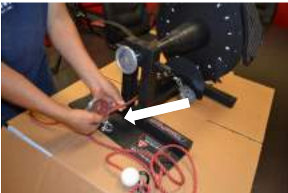
5. Pull rope through two columns.
