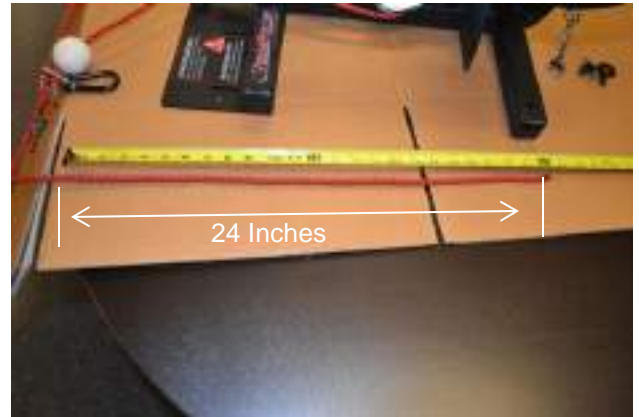
7. Measure off 2 feet of rope. This is needed for knot assembly. Tilt PVP back up into standard position.
